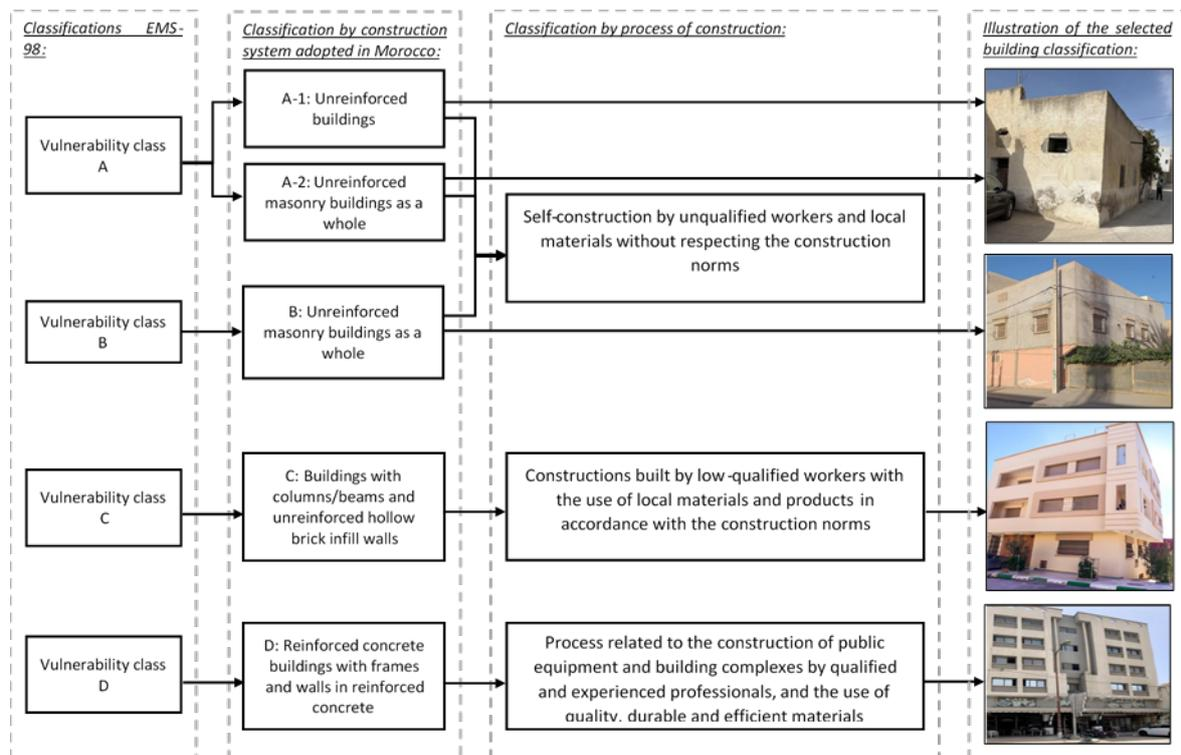
Figure 2. Synthetic schema of the classification of buildings in Morocco.
