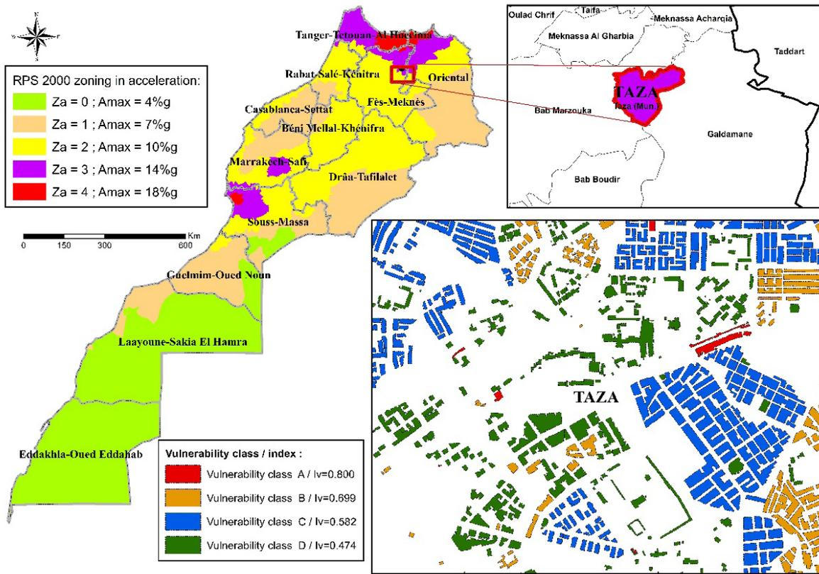
Figure 3. Spatial representation of seismic vulnerability classes of buildings in the Taza urban area.
