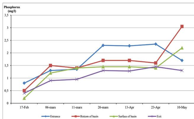
Figure 9. Spatio-temporal trends of phosphorus concentration in water samples collected from four locations of treatment station during study period.
