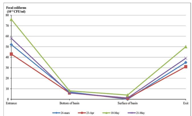
Figure 14. Spatio-temporal trends of number of fecal coliforms in water samples collected from four locations of treatment station during study period.
