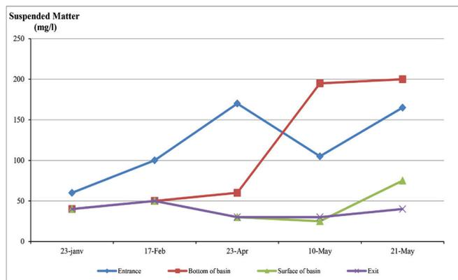
Figure 8. Spatio-temporal trends in suspended matter concentration of water samples collected from four locations of treatment station during study period.
