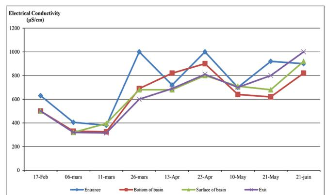
Figure 4. Spatio-temporal trends in Electrical Conductivity values of water samples collected from four locations of treatment station during study period.
