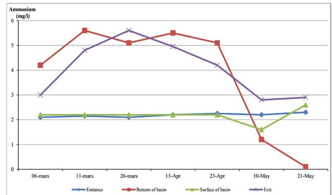
Figure 10. Spatio-temporal trends of ammonium concentration in water samples collected from four locations of treatment station during study period.
